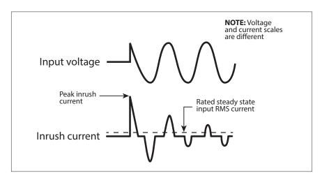
Fig 4.1: Inrush current in an SMPS
