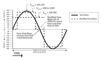
Fig. 2.1: Pure and Modified Sine Waveforms for 230 VAC, 50/60 Hz
