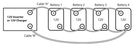
Fig 7.3: Parallel Connection
