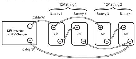
Fig. 7.4: Series-Parallel Connection
