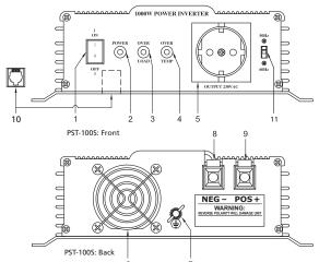
Fig. 6.2: Layout of PST-100S-12E, PST-100S-24E
