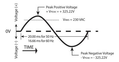
Fig. 5.1: 230 VAC, 50/60 Hz Pure Sine Waveform
