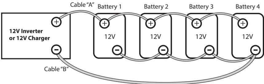
Fig 7.3: Parallel Connection
