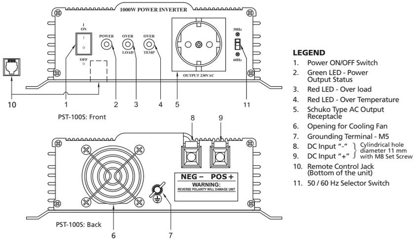
Fig. 6.2: Layout of PST-100S-12E, PST-100S-24E
