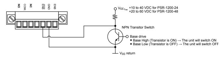
Fig 5.5 2-Wire Remote Control ON / OFF using ENB and GND Terminals and External Transistor Switch
