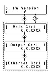
Group 5 of Main Menu "FW Version" leads to 3 Sub-Menu screens that provide Firmware (FW) Version Nos. for the following 3 Micro-Controllers (see Fig 10.2):
