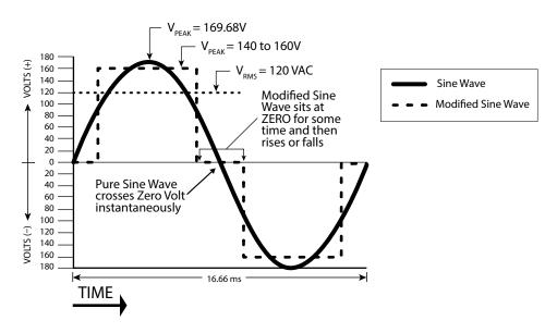
Fig. 2.1: Pure and Modified Sine Waveforms for 120 VAC, 60 Hz
