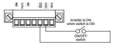
Fig 5.3 2-Wire Remote Control ON / OFF using ENB and GND Terminals
