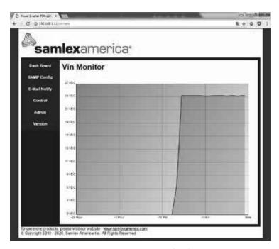
Fig 13.4 DC Input Voltage (Vin) Monitor
