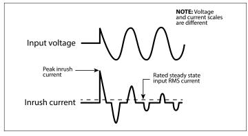
Fig 4.1: Inrush current in an SMPS
