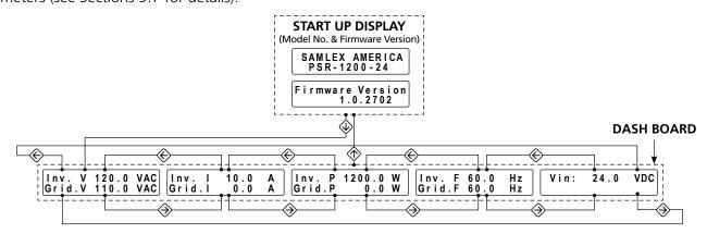
Fig 9.1: Startup Display and Dashboard (extract from Fig 10.1)
