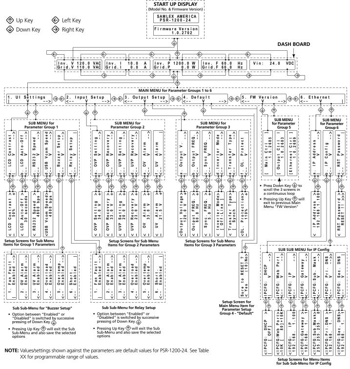
Fig 10.1 Menu Map for Programmable Operating Parameters
