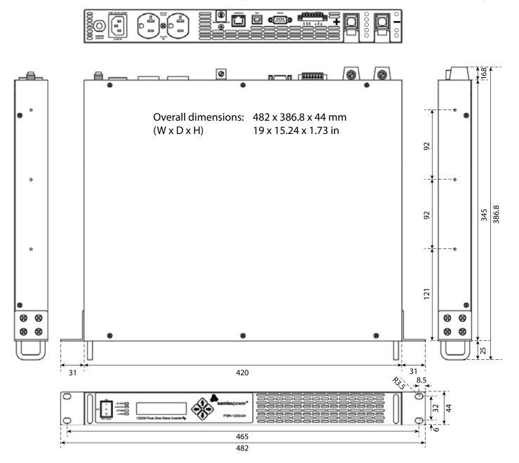
Fig. 8.1: PSR-1200-24 & PSR-1200-48 - Overall Dimensions & Mounting Arrangement
