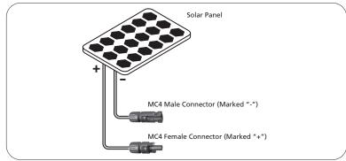
Fig 3. Solar panel connecting wires with MC4 Connectors
