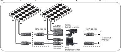
Fig. 5. Connecting two solar panels in parallel that are separated by an extended distance
