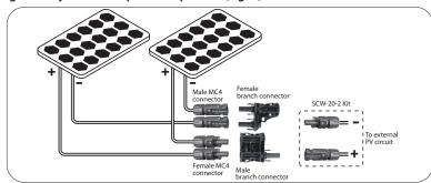
Fig. 4. Connecting two adjacent solar panels in parallel
